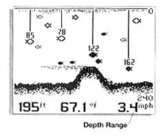
When "Manual" range is used. the unit no longer adjusts the Depth Range to the most appropriate range for bottom display. Often, the bottom may not be visible on-screen. The digital depth readout always determines the depth of the bottom, even if it is not visible on-screen.
